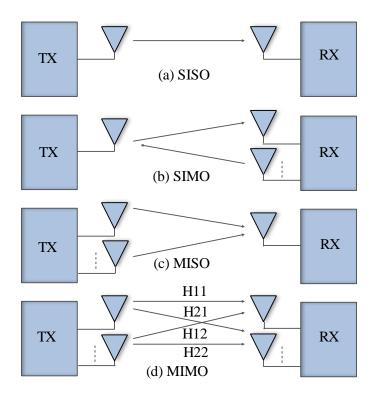
Figure 3.2 Various types of wireless communication.
