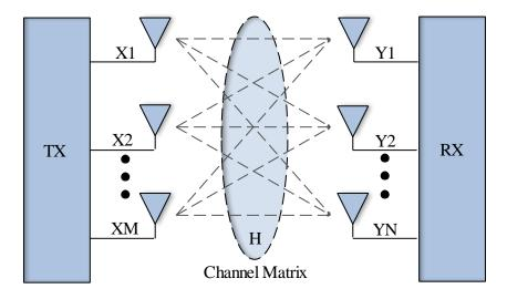
Figure 3.3 Annotative illustration of a MIMO system
