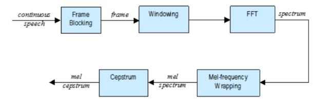
Figure 1.0: Block Diagram of MFCC Processor
