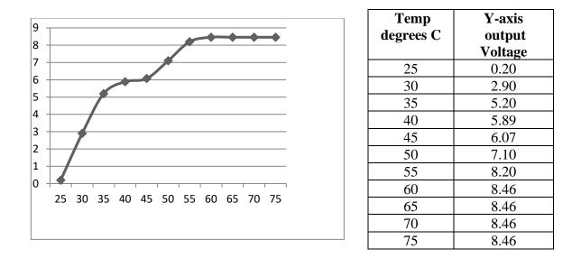
Figure 5.3 Relationship between source temperature and voltage.
