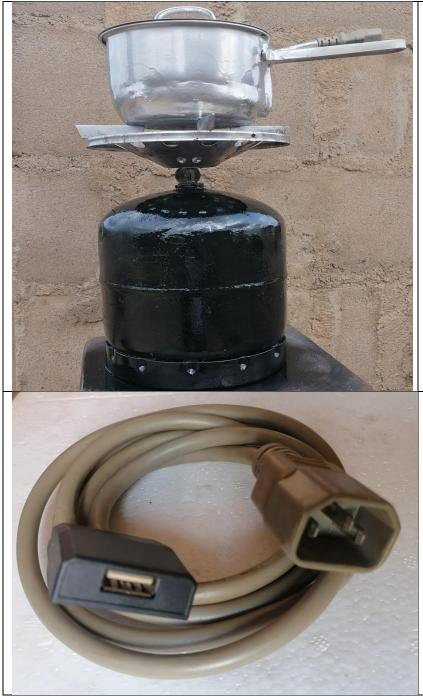
Pot model of cooking heat-based cell phone battery charger. Works with any type of cooking fire arrangement.
