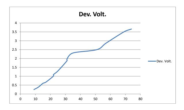
**Figure 2c:** showing voltage generation with respect to temperature difference.
