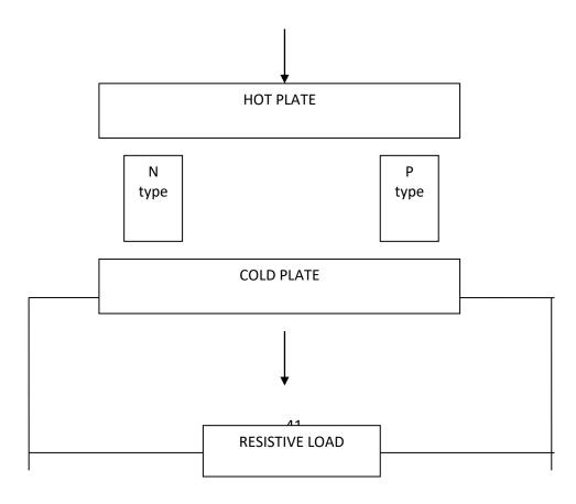
Figure 4a. Schematic diagram of the Thermoelectric Couple.
