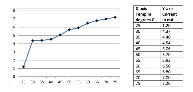
Figure 8:-Relationship between temperature change and current.
