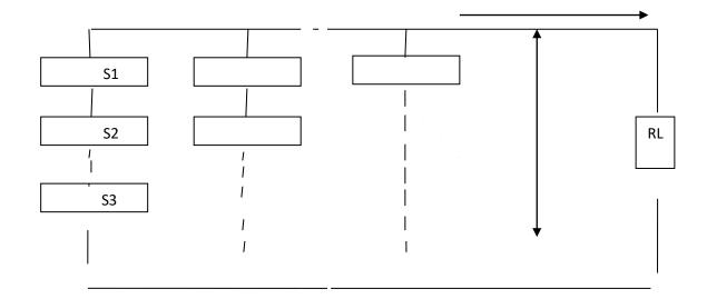
**Figure 5.** Our Thermoelectric Generator with a Series-Parallel Arrangement of Modules.
