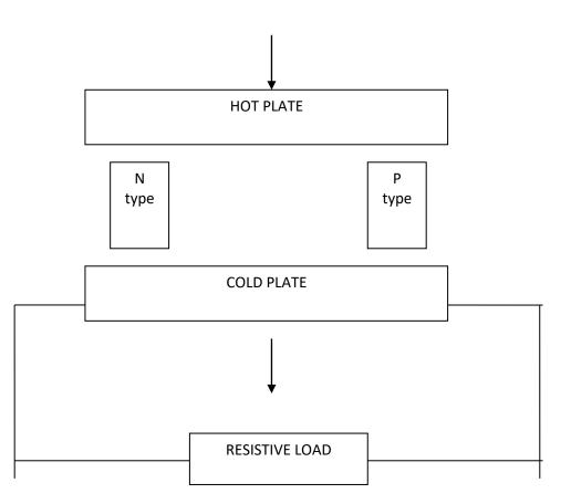
Figure 4. Single Thermoelectric Couple (Th > Tc).
