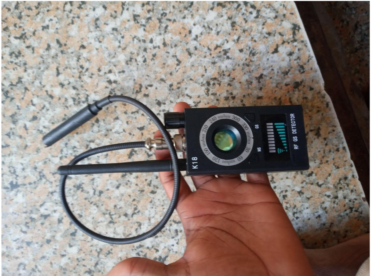
**Figure 2: Signal Frequency Detector**
