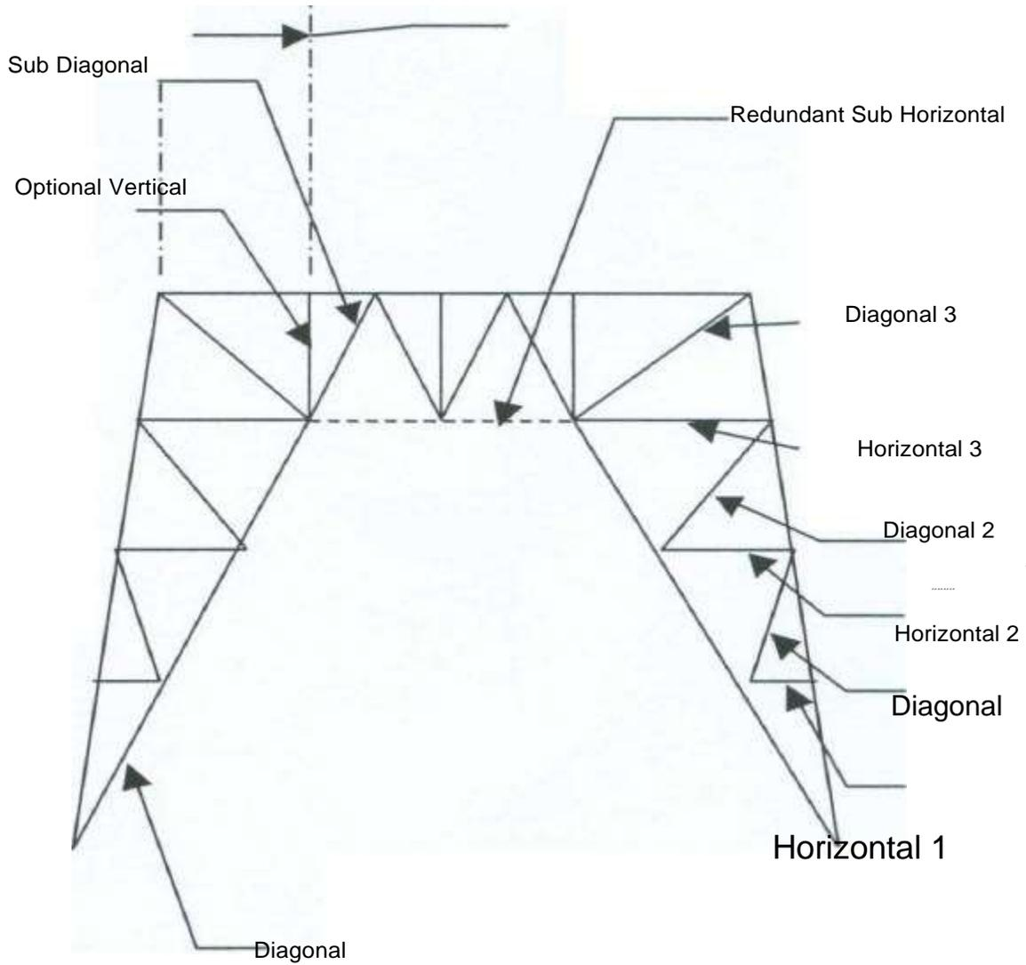
**Figure 2.8 Portal Bracing**
