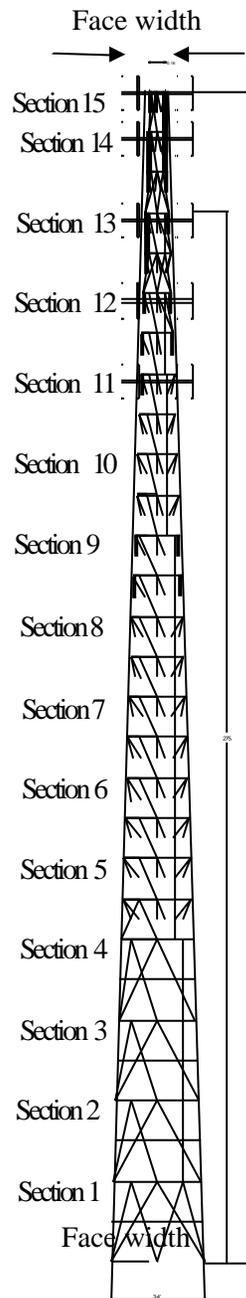
This represents a generalized design of a 15 section, 6m length per section tower.
