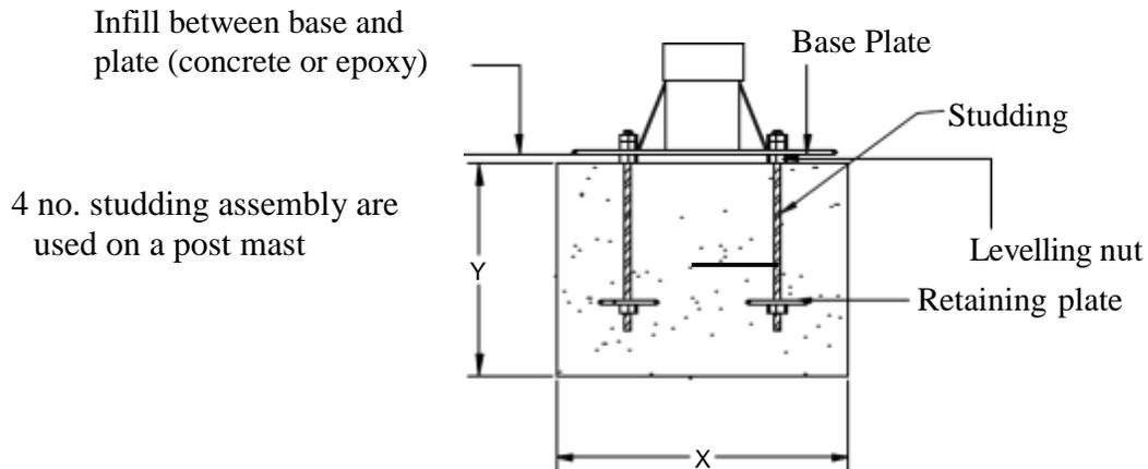
Dimensions of X and Y are dependent on soil conditions, dead weight of mast and wind loading
