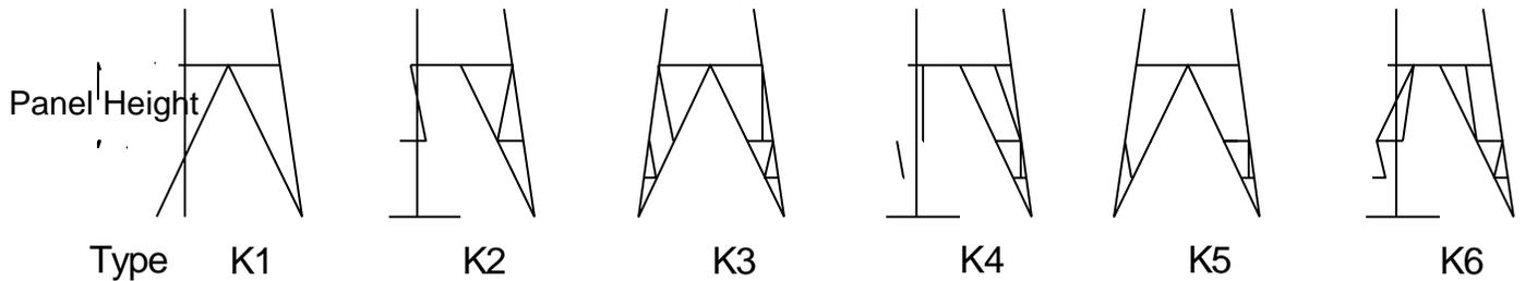
**Figure 2.1 – Bracing Types**
