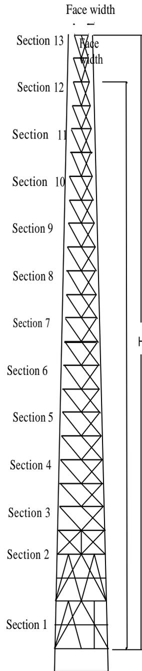
Generalized prototype design of a 13 section, 6m lengths per section tower.
