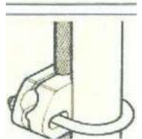
*Typical clamps for installation of earth tapes*
