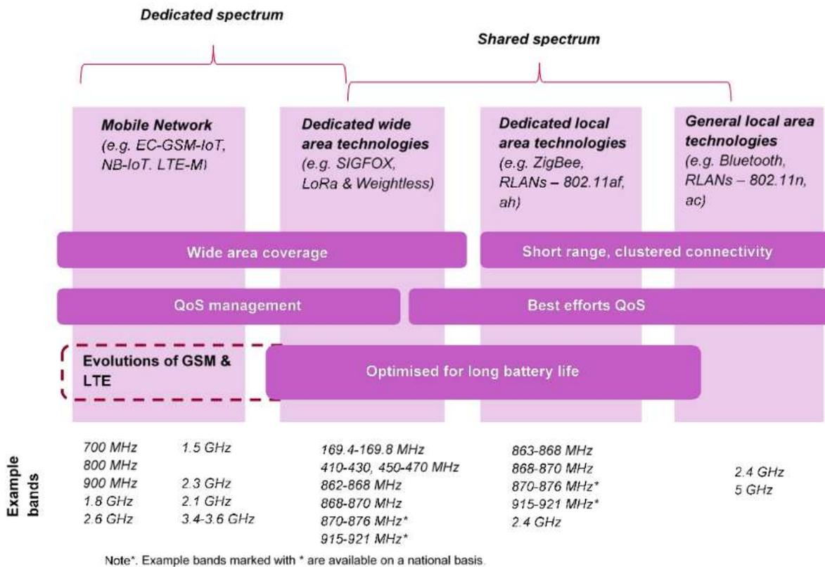
The use of low bands (below 1GHz) should be the basic goal for mobile operators when offering NB-IoT solutions. For example, the NB-IoT chipset is fully supported in APT700, along with other IMT bands below 1 GHz, and there are considerable and compelling benefits in deploying APT 700 including enhanced indoor coverage, wider coverage that extends to suburban and rural areas, higher speeds and improved IoT deployments.
