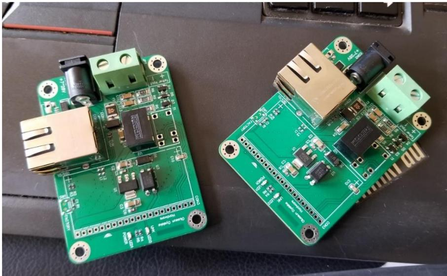
Figure 5: The prototype (PCB, without transformer, with transformer)
