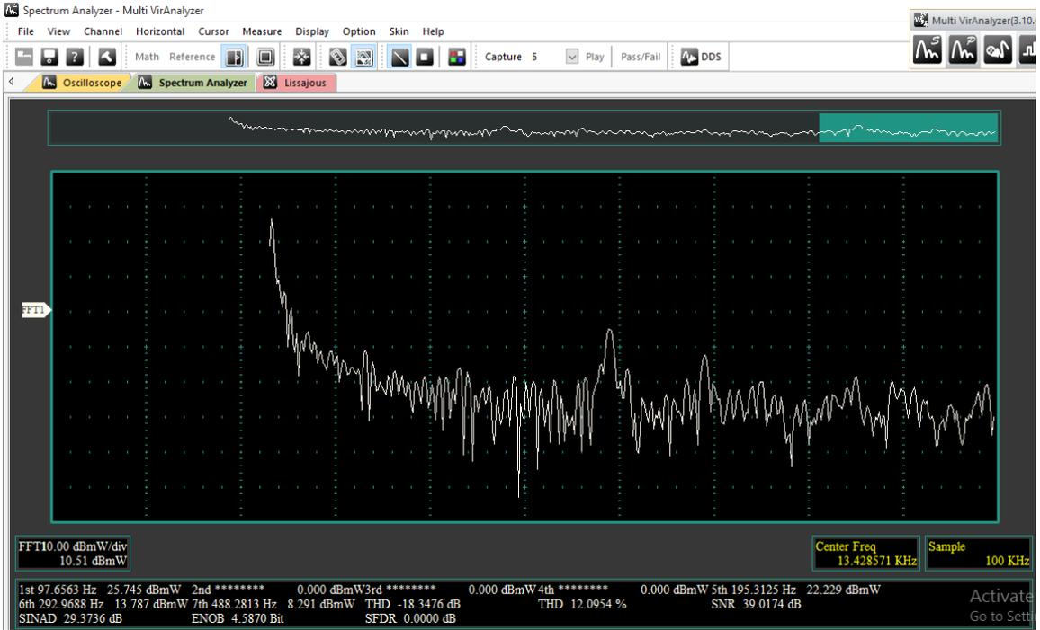
Figure 25: Center Carrier frequency of lower range 13KHz (On LV Line) with harmonic
