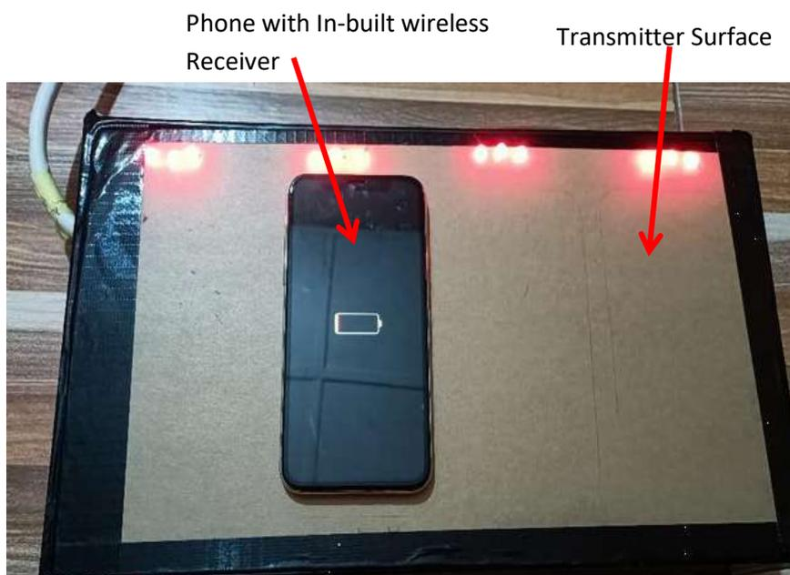
Fig 50: An Energised four (4) Compartment Transmitter prototype charging a phone with an inbuilt wireless receiver (iphone 11 promax) .
