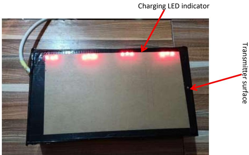
Fig 49: An Energised four (4) Compartment Transmitter prototype
