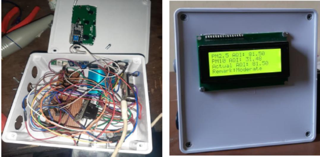
Figure 3.18: Complete package of the FWSN
