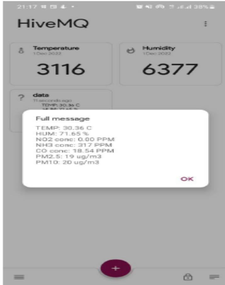
Figure 4.6: Display showing the real-time harvested data on the display of the FWSN
