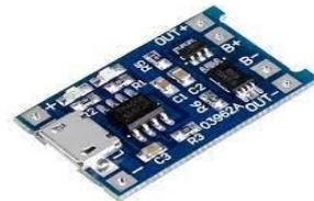
Fig. 1.5 Tp4065 Battery Charging Module
