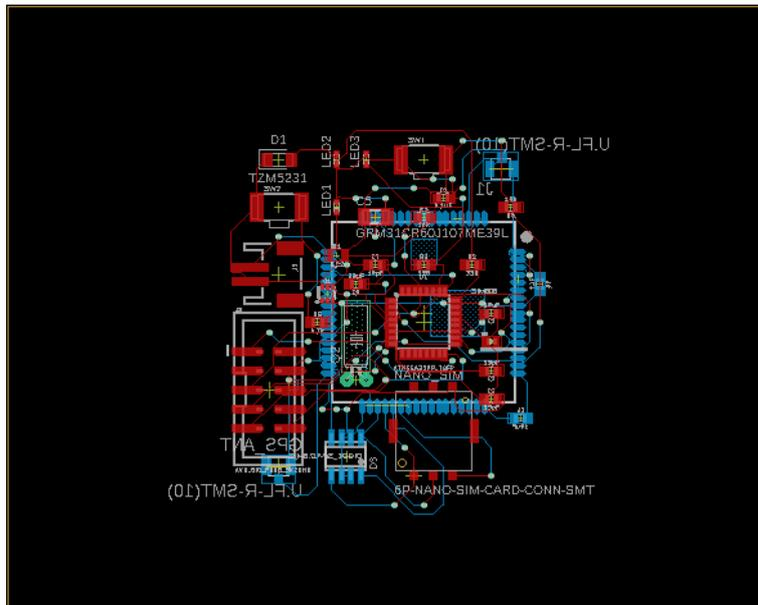
**Figure E.3: PCB Design for the eBand**
