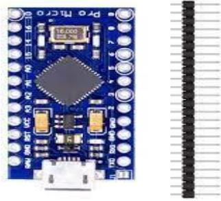
Fig. 1.3: Arduino Pro Micro
