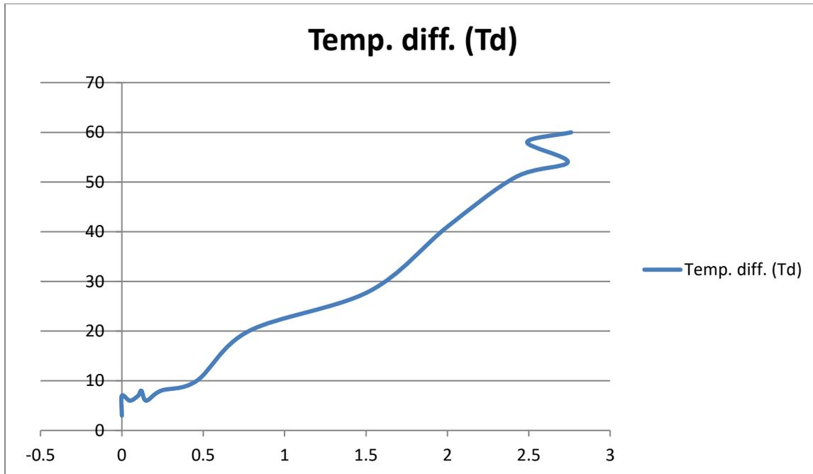
**Figure 3.15:-** Relationship developed voltage and temperature difference at ambient temperature of 36 C.
