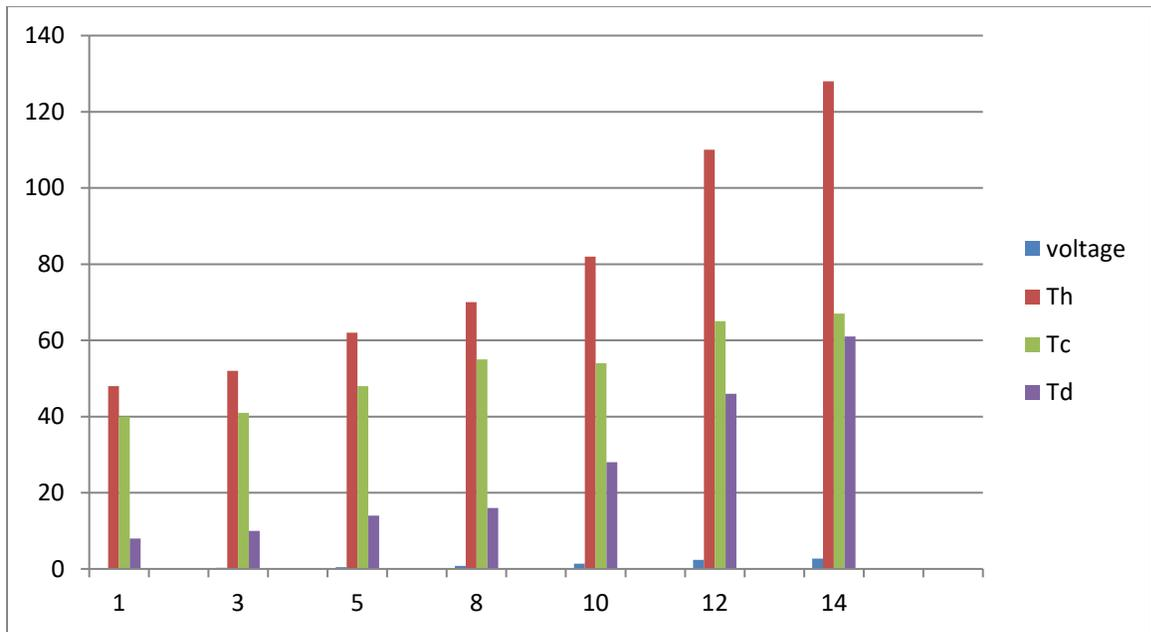
**Figure 5.12:-** Relationship developed voltage and temperature difference at ambient temperature of 33 C.
