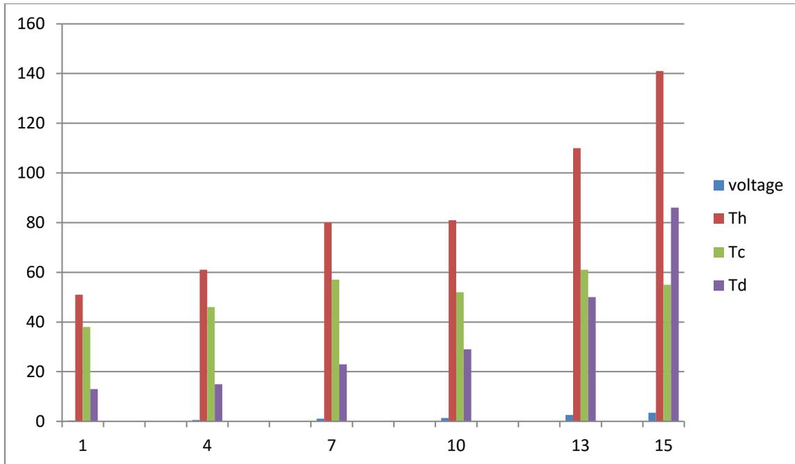
**Figure 5.10:-** Relationship developed voltage and temperature difference at ambient temperature of 32 C.
