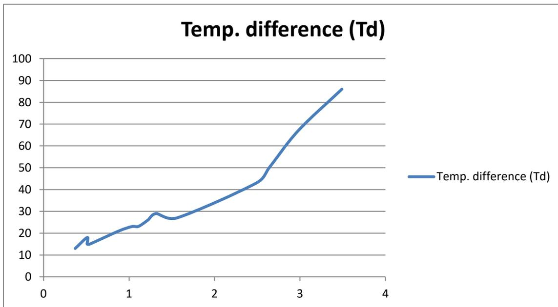
**Figure 5.11:-** Relationship developed voltage and temperature difference at ambient temperature of 32 C.
