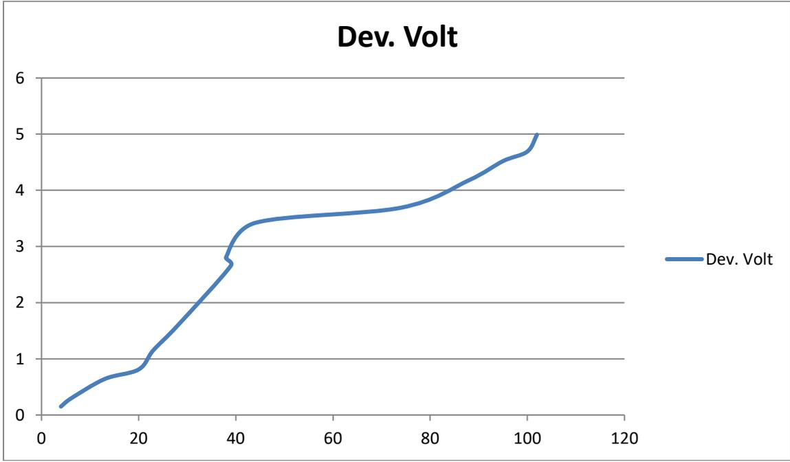
**Figure 1c.** Change in developed voltage with temperature diff.
