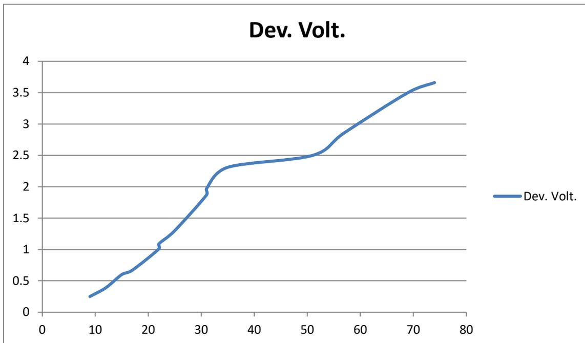
**Figure 2c:** showing voltage generation with respect to temperature difference.
