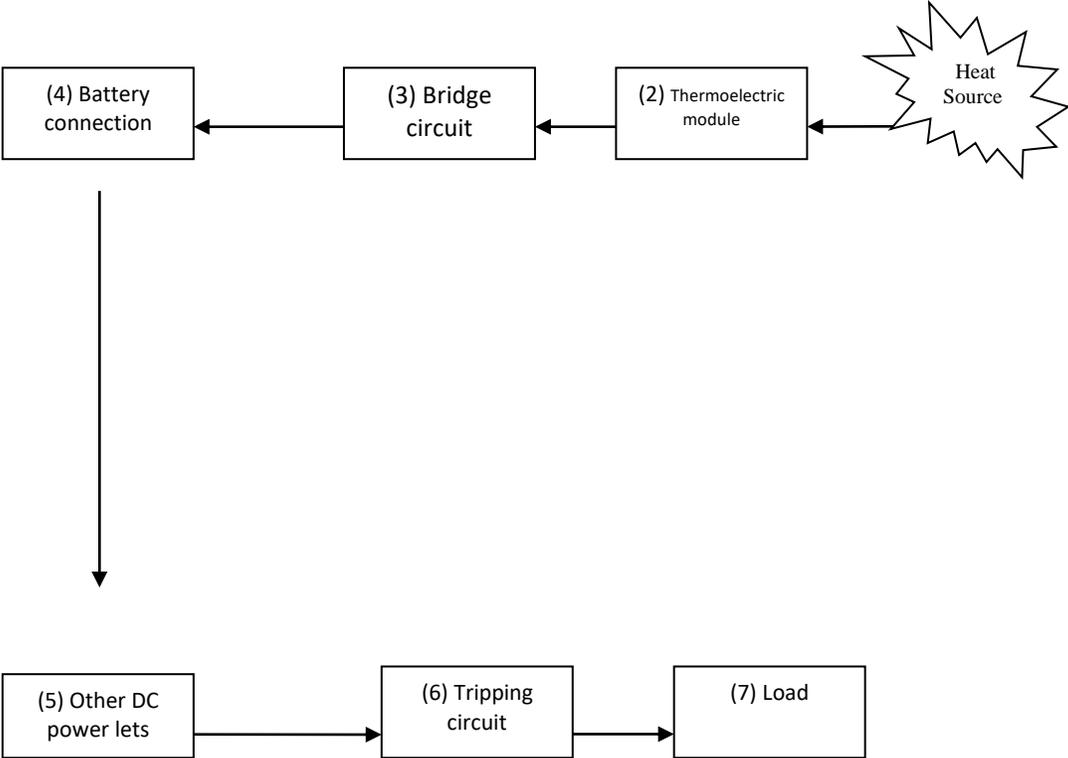
**Figure 2:** Block diagram of the 12volts, 1.5Amp cell phone charger.
