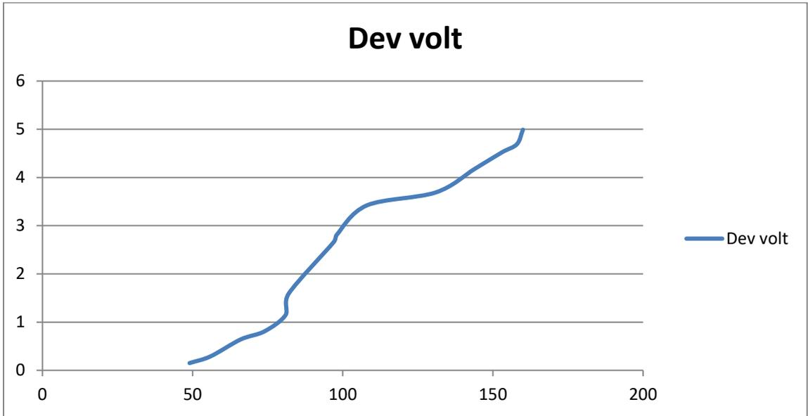
**Figure 1b** Change in developed voltage with hot side temperature.
