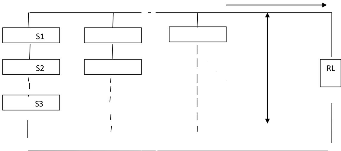
**Figure 5.** Our Thermoelectric Generator with a Series-Parallel Arrangement of Modules.
