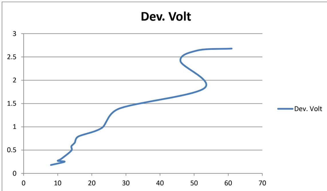
**Figure 4c:** showing voltage generation with respect to temp change.
