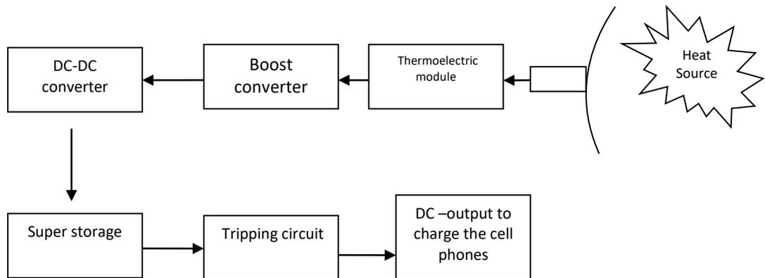
**Figure 3:** Block diagram of the 6volts, 1.5Amp cell phone charger.
