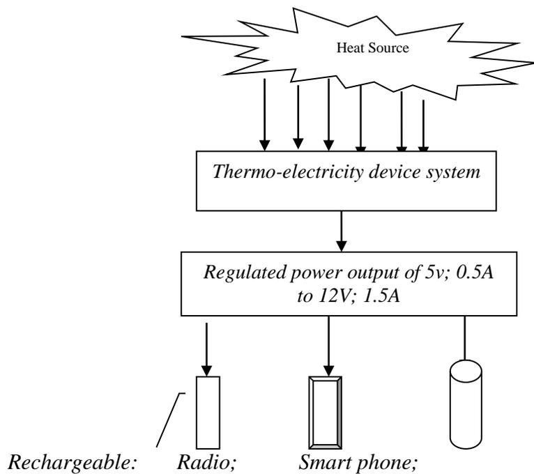
Figure 1: Operational arrangement of heat-to-electrify charger.
