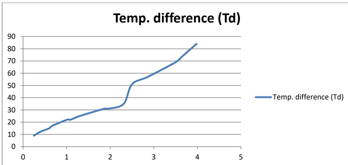
**Figure 5.9:-** Relationship developed voltage and temperature difference at ambient temperature of 30 C.
