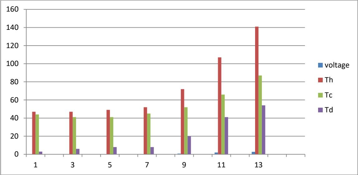
**Figure 5.14:-** Relationship developed voltage and temperature difference at ambient temperature of 36 C.
