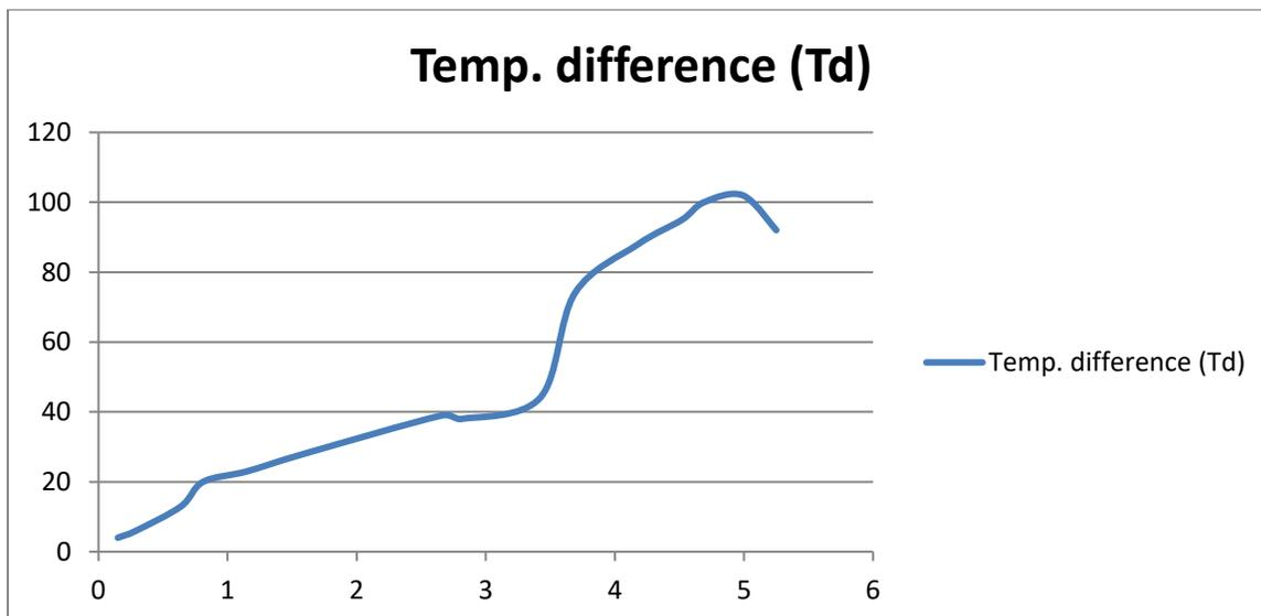
**Figure 5.7:-** Relationship developed voltage and temperature difference at ambient temperature of 29 C.
