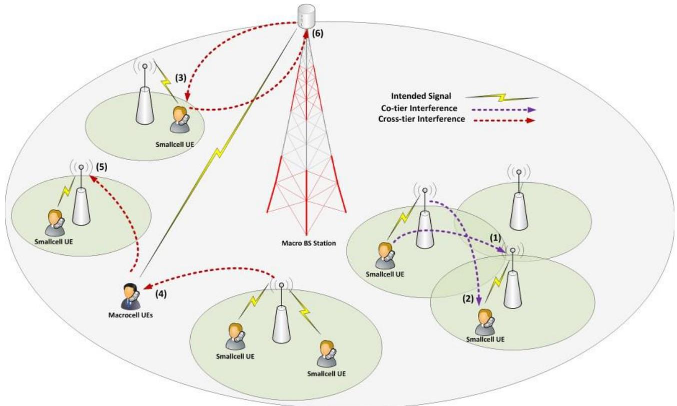
Figure 1.1: Different cases of inter-tier and intra-tier interference in 5G Heterogeneous Network
