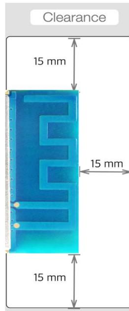
Figure 4.4: Meandered Planar Inverted-F Antenna
