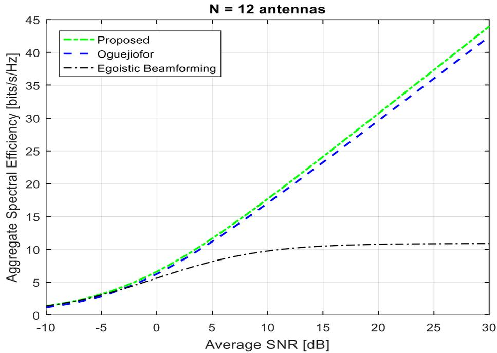
Fig. 3.8: Aggregate Spectral efficiencies achievable at different SNR for  $N=12$ ,  $Kr=4$ .
