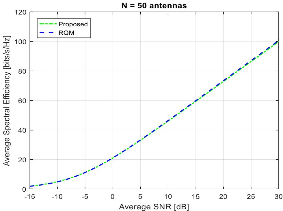
Fig. 3.6: Average Spectral efficiencies achievable at different SNR for  $N=50$ ,  $m=9$
