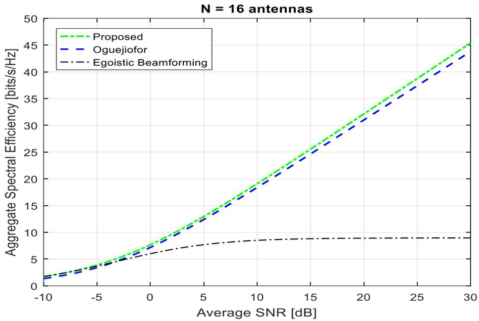
Fig. 3.9: Aggregate Spectral efficiencies achievable at different SNR for  $N=16$ ,  $Kr=4$
