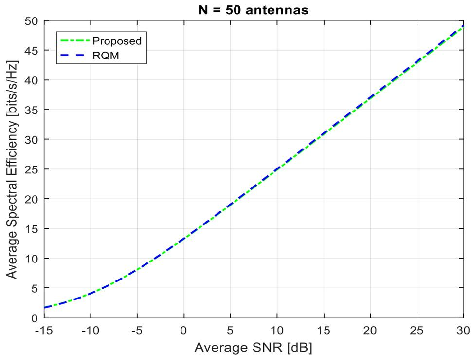
Fig. 3.4: Average Spectral efficiencies achievable at different SNR for  $N=50$ ,  $M=4$
