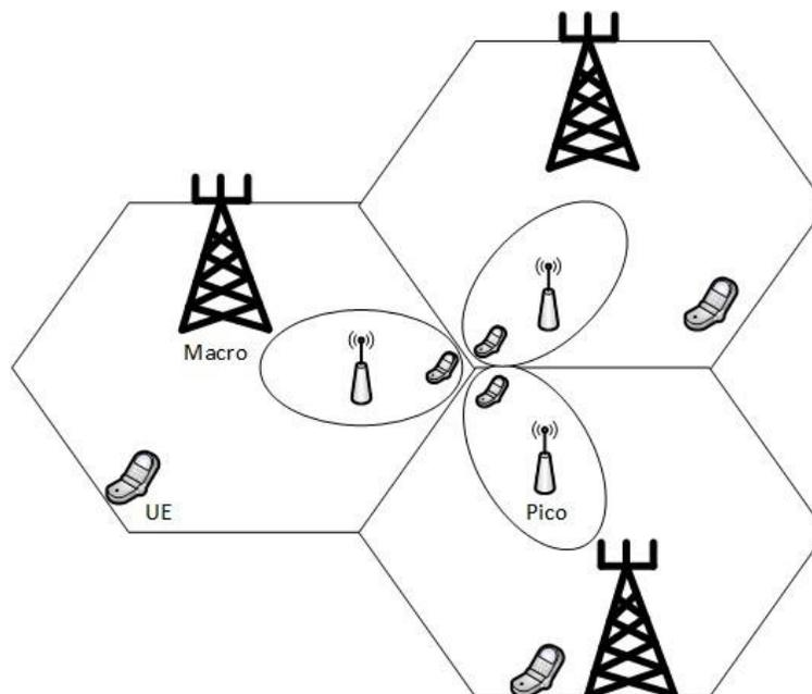
Figure 1.2: Downlink 5G heterogeneous system with Pico cells in the coverage area of MBS
