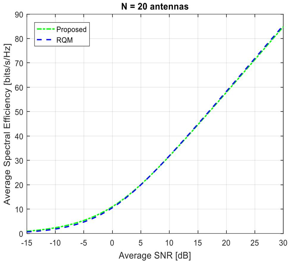
Fig. 3.5: Average Spectral efficiencies achievable at different SNR for  $N=20$ ,  $M=9$
