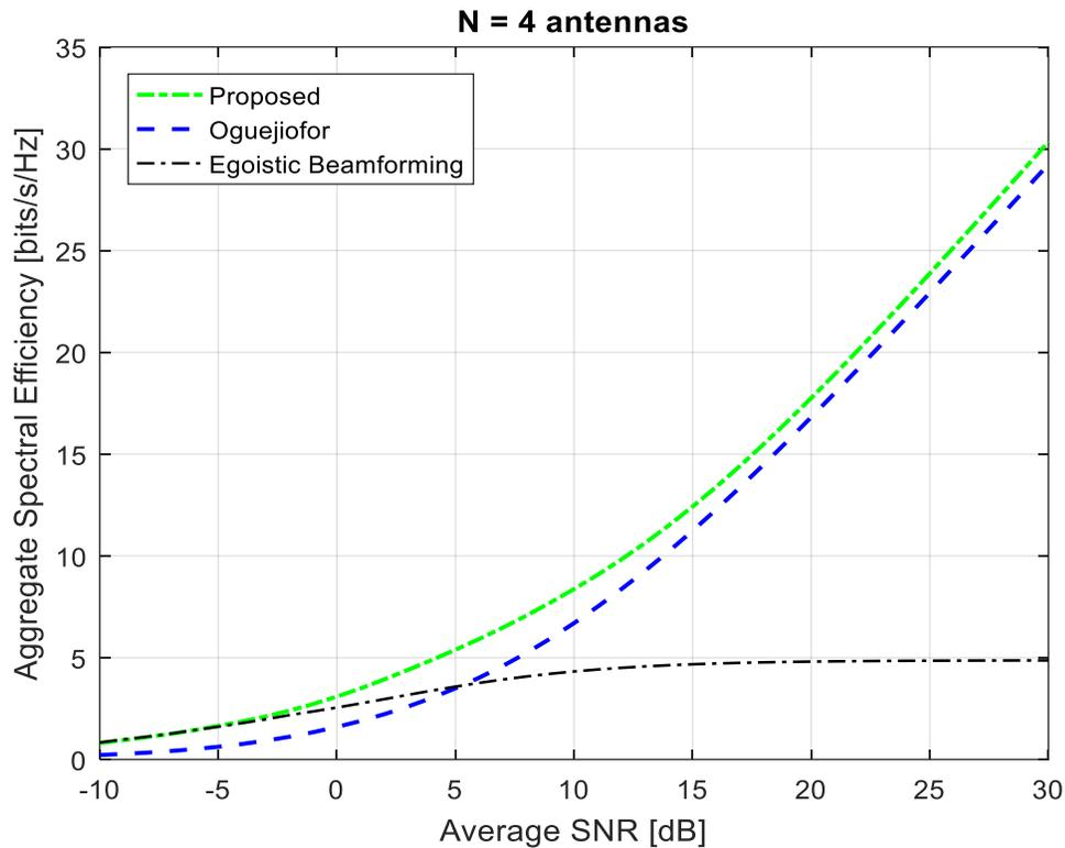
Fig 3.7: Aggregate Spectral Efficiency as a function of SNR for different beamformers
