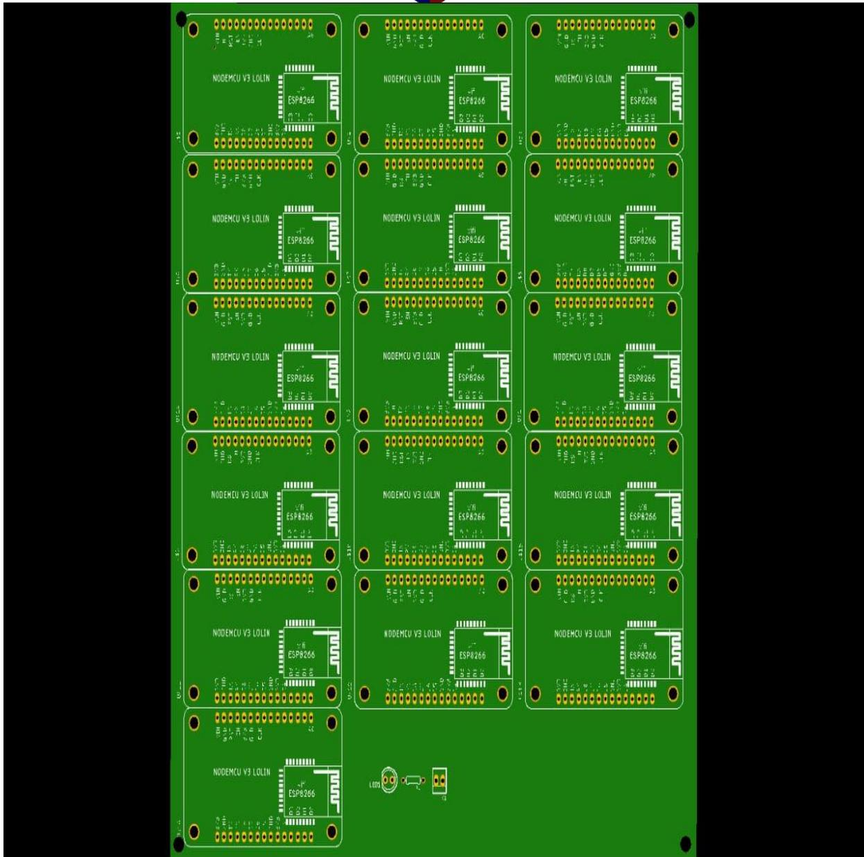
Figure 4.7: Multi-antenna System Custom PCB Design
