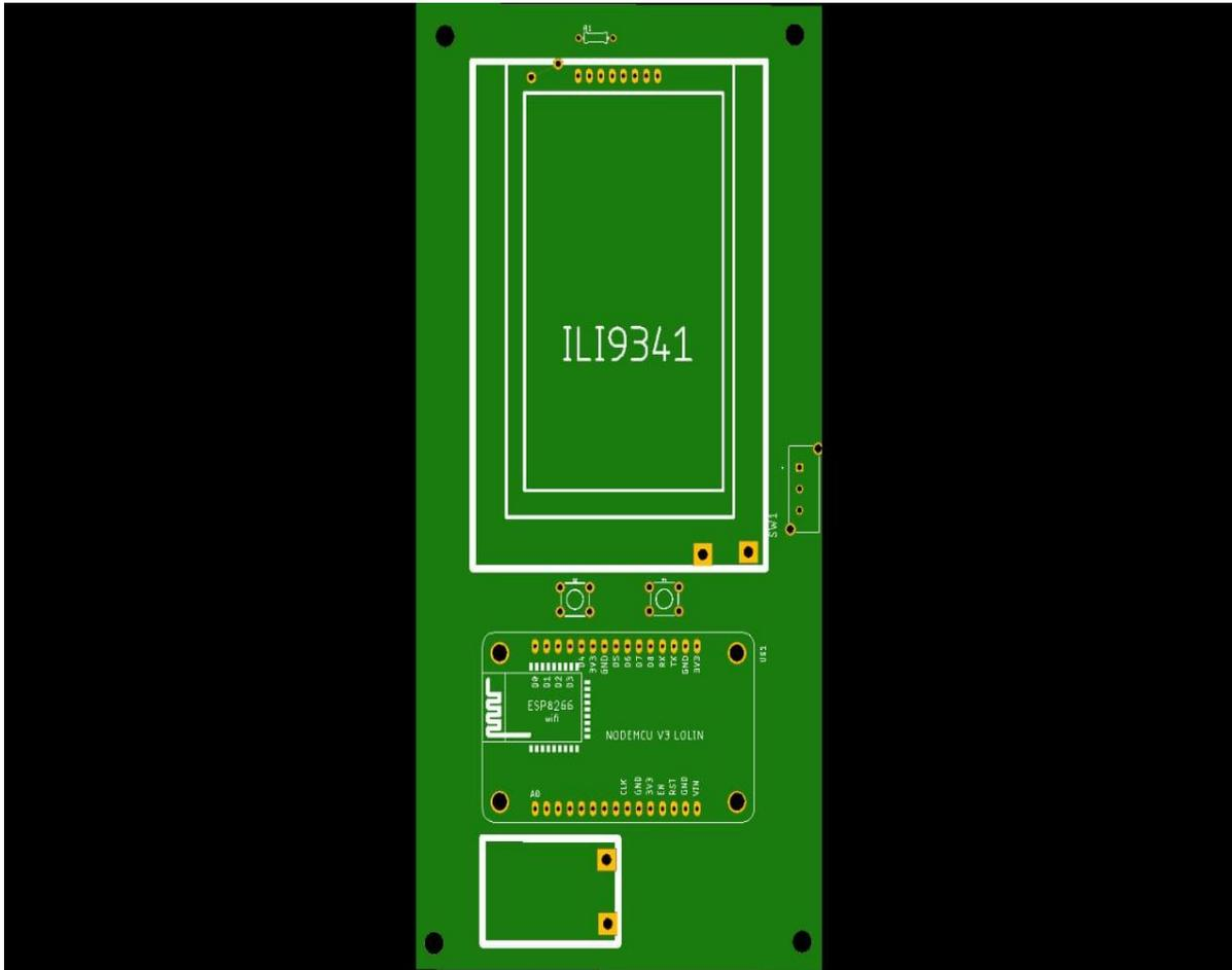
Figure 4.15: The PCB Design of the Receiver Unit
