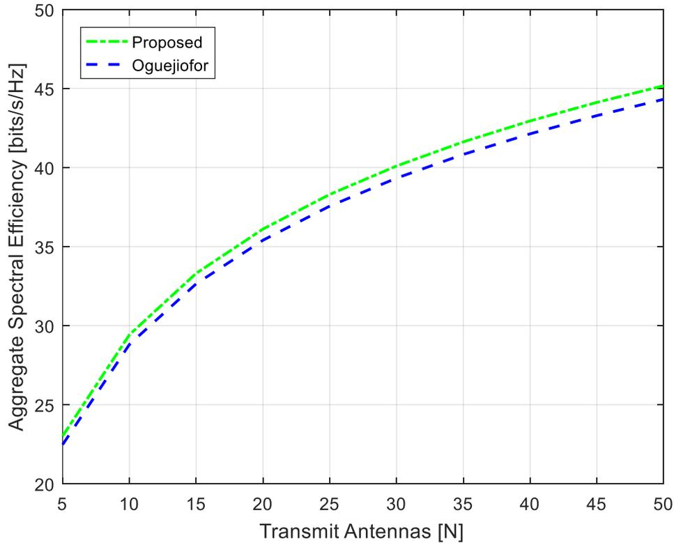
Fig. 3.12: Aggregate spectral efficiency at different transmit antenna for  $SNR = 10\text{dB}$
