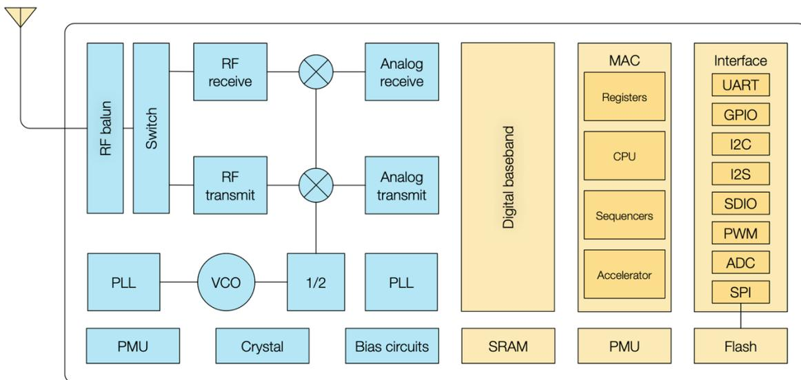
Figure 4.1 Block diagram of ISM43340 Chipset
