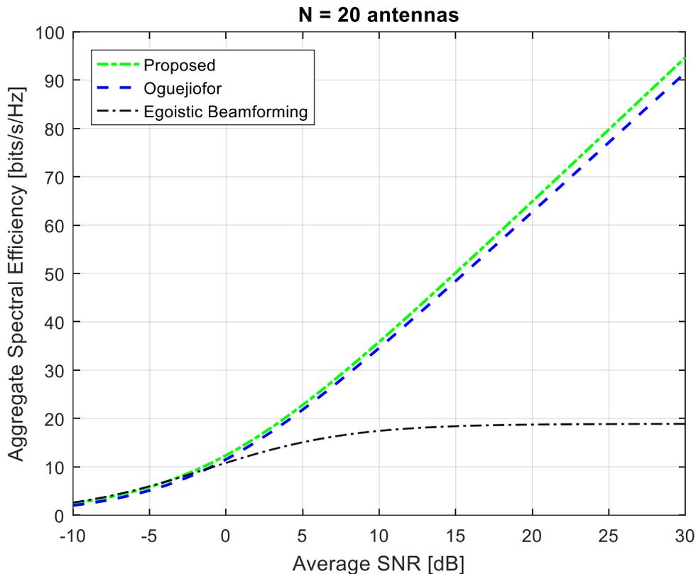
Fig. 3.11: Aggregate Spectral efficiencies achievable at different  $SNR$  for  $N=20$ ,  $Kr=9$ .
