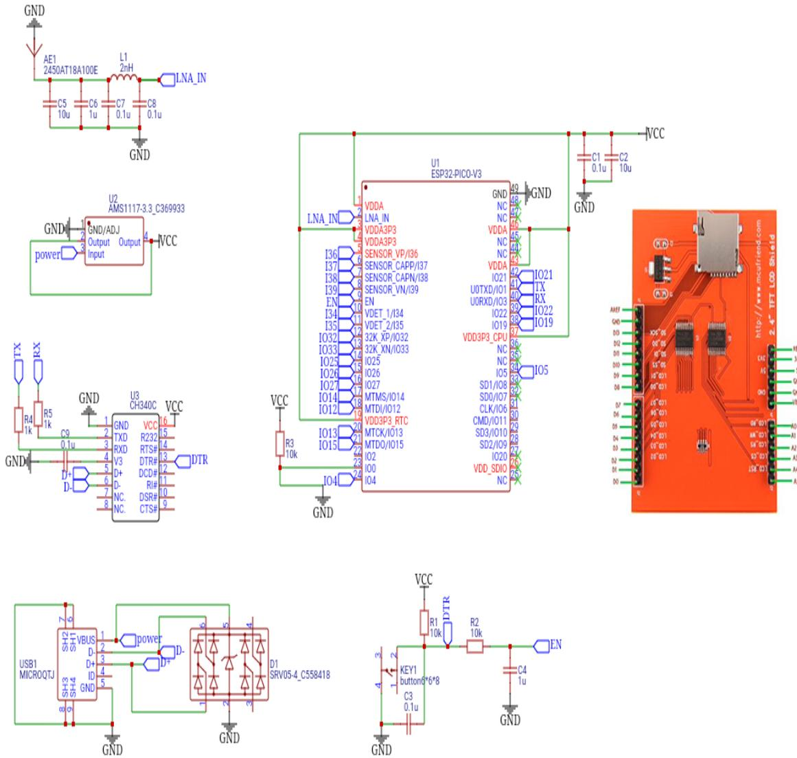
Figure 4.17: Schematic Circuit Diagram for the Network Visualizer
