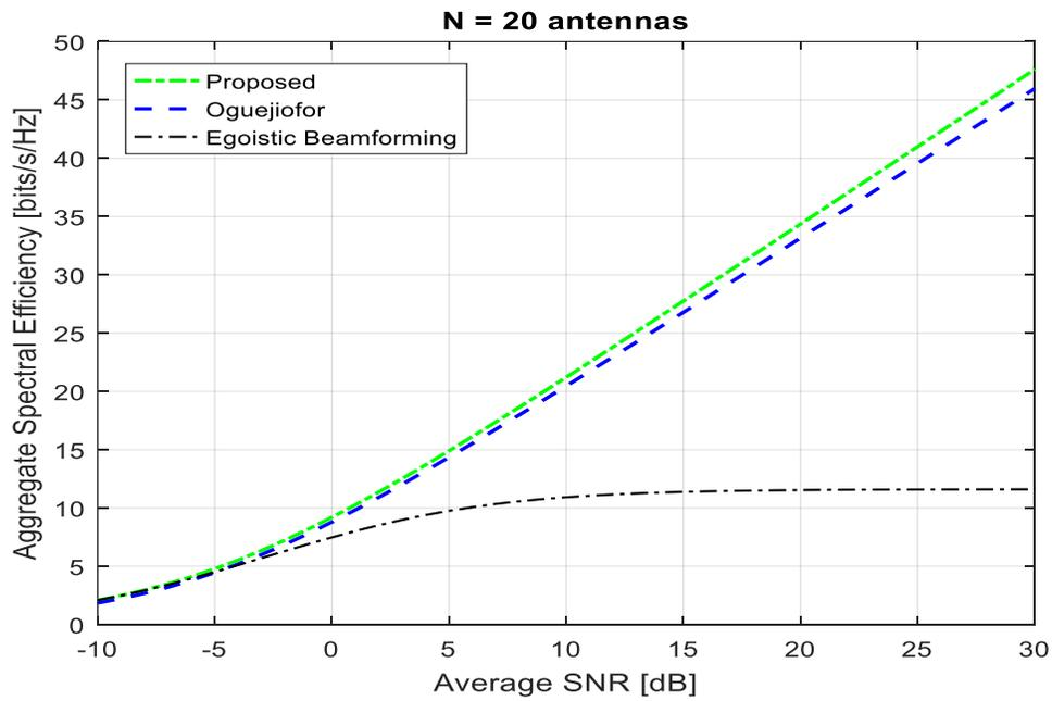
Fig. 3.10: Aggregate Spectral efficiencies achievable at different SNR for  $N=20$ ,  $Kr=4$
