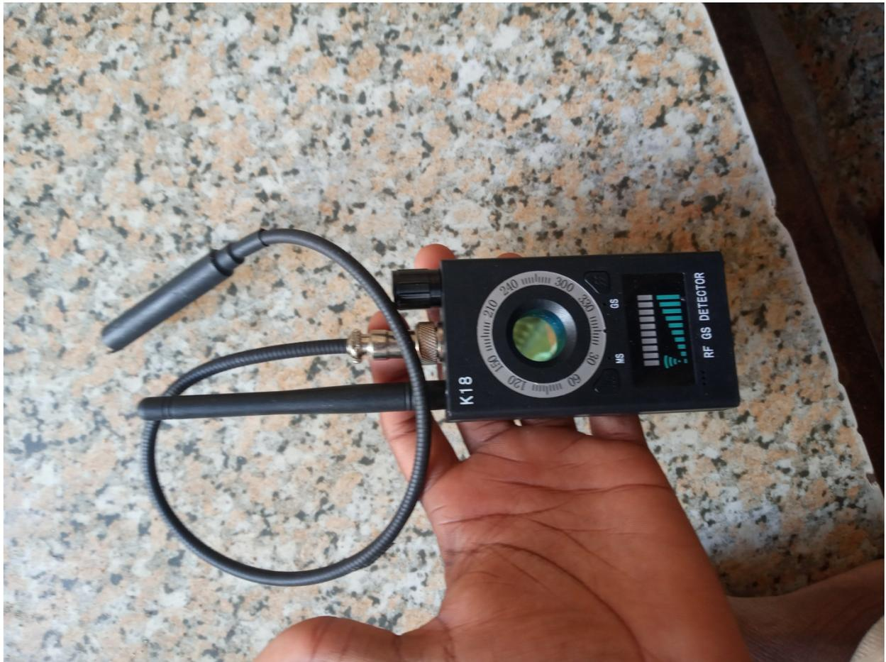
**Figure 2: Signal Frequency Detector**
