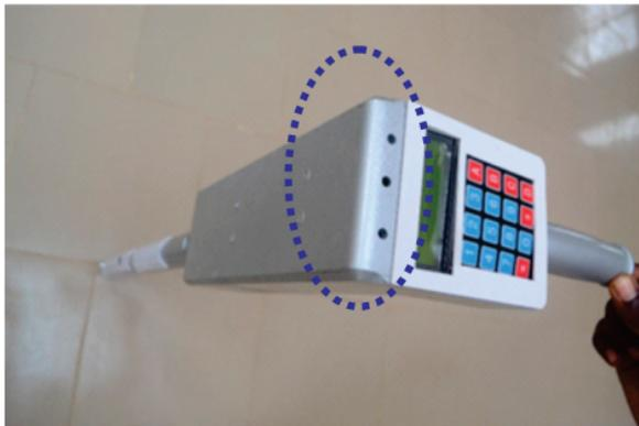
Figure 1.3: MCEWS Fall Detection Unit
