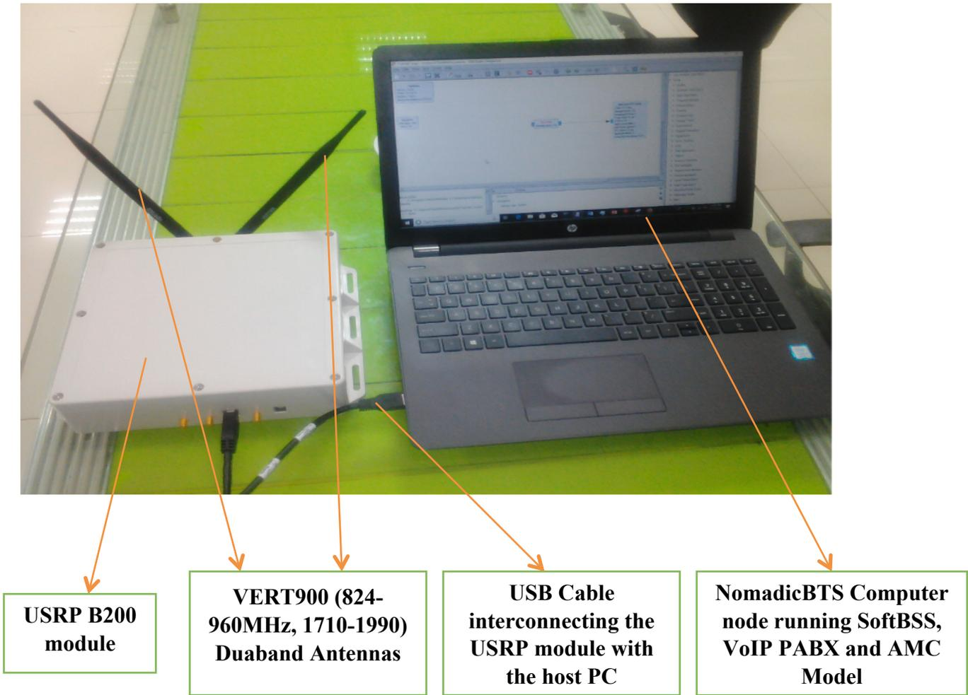
Figure 4.0: NomadicBTS Prototype Showing Interconnection of USRP-B200 with the host PC
