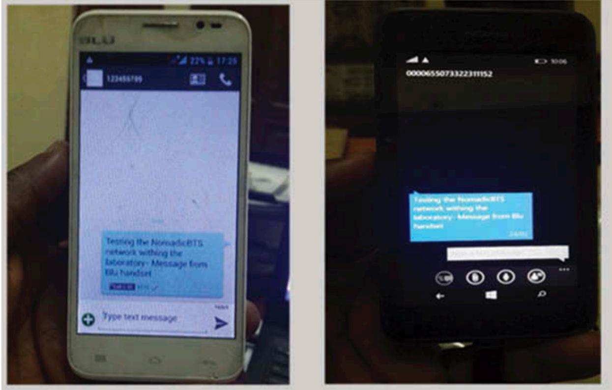
Figure 21.0: Successful SMS Communication Between the Test Phones on the NomadicBTS Prototype Cell.
