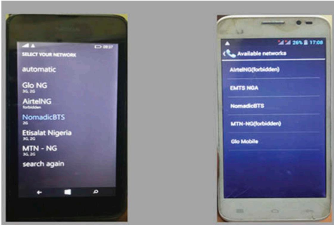
Figure 20.0: Successful Registration of Test Phones on the NomadicBTS Prototype Cell
