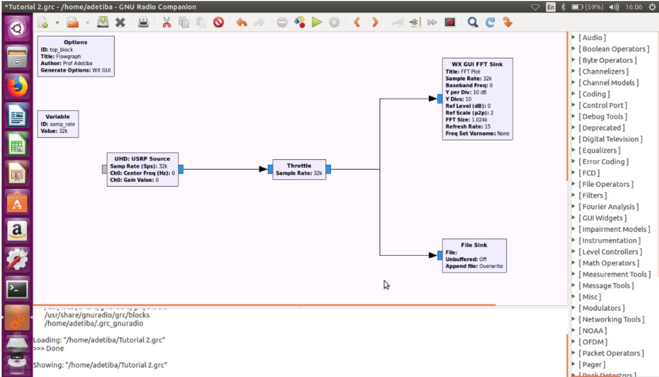
Figure 13.0: Flowgraph for Modulated Signal Capturing
