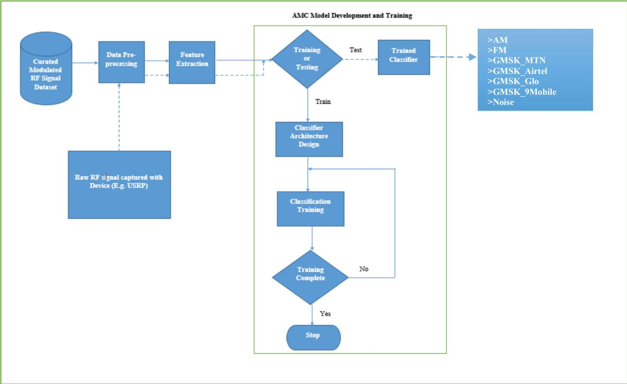
Figure 10.0: Flowchart for Intelligent Spectrum Sensing Implementation with AMC Model
