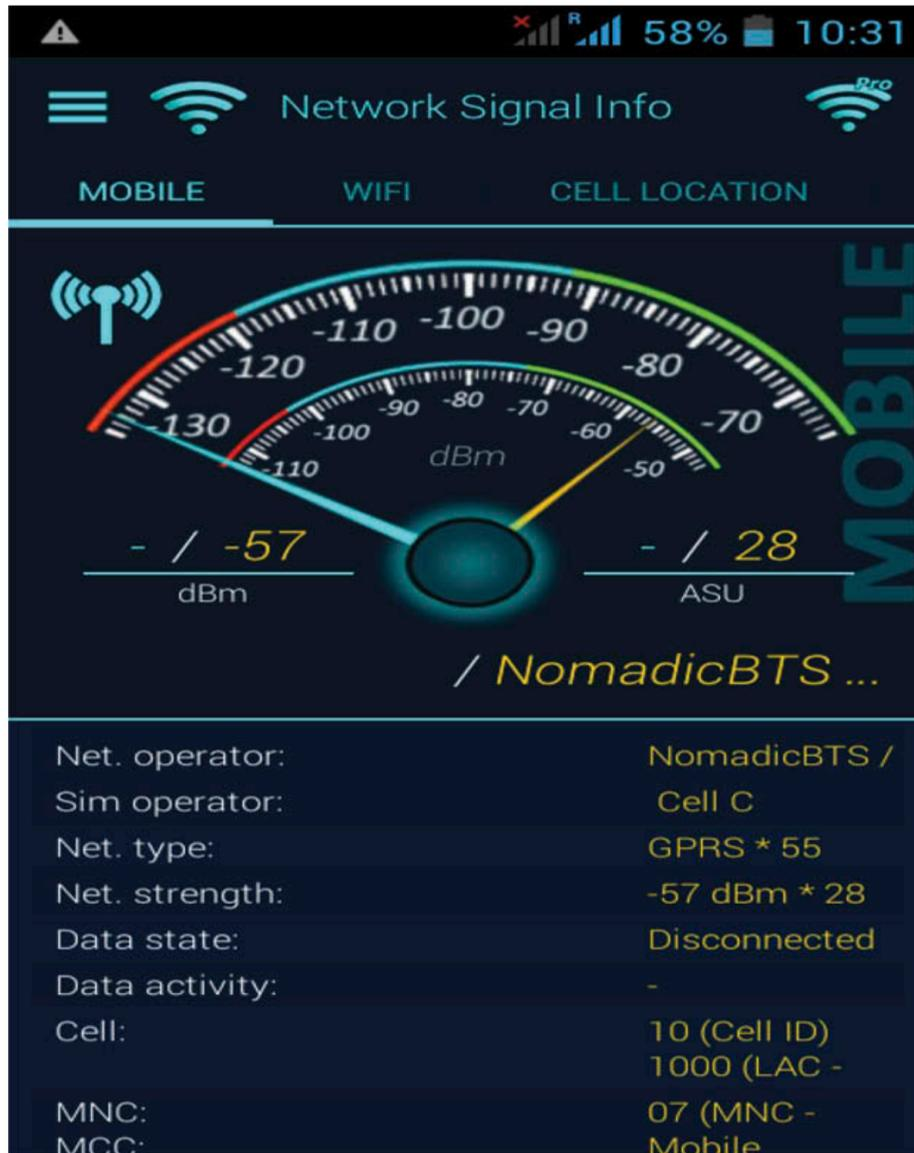
Figure 19.0: Signal Measurement on a Test Mobile Phone at Close Proximity to the NomadicBTS Prototype Cell
