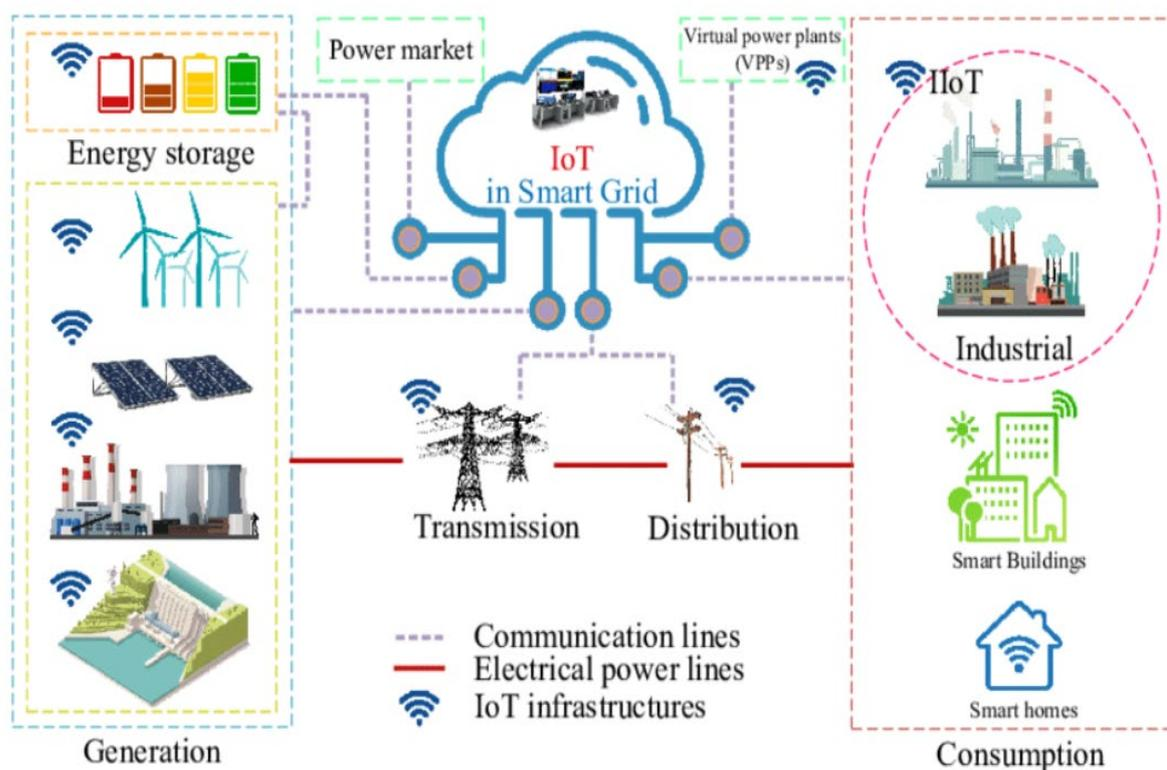
**Figure 14:** The paradigm of IoT in smart electricity grids; Source: [www.researchgate.net](http://www.researchgate.net)
