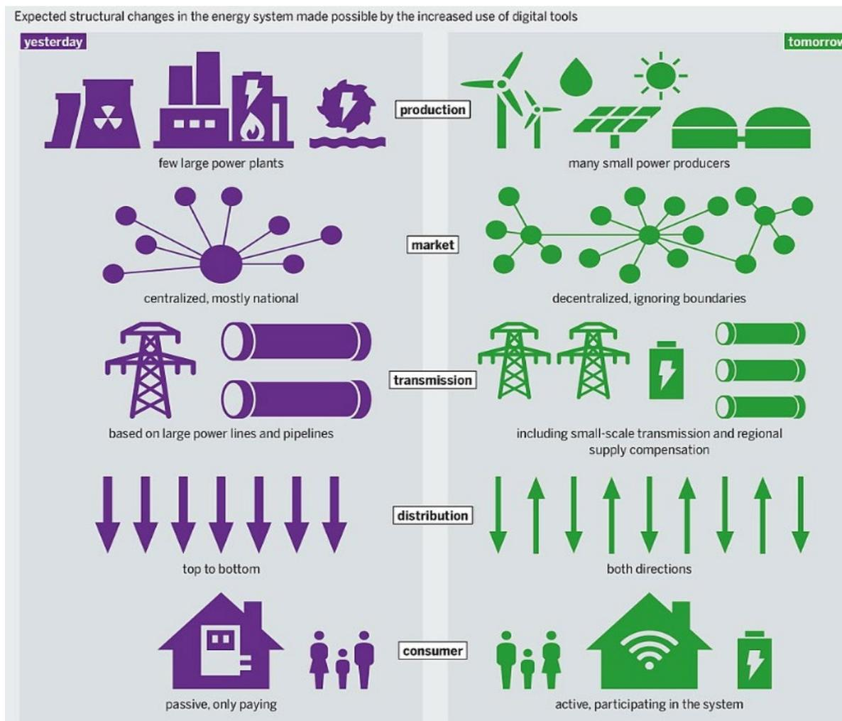
**Figure 15:** Characteristics of a smart grid (right) versus the traditional system (left);
